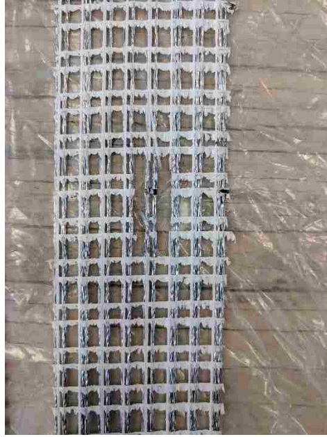
Figure 3.23. Location of strain gauge without fiberglass backing
