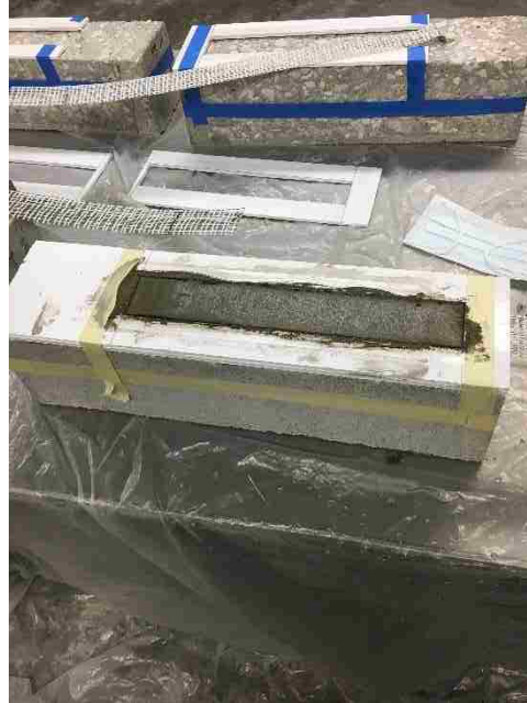
Figure 3.12. Final (external) matrix layer applied over steel fibers
