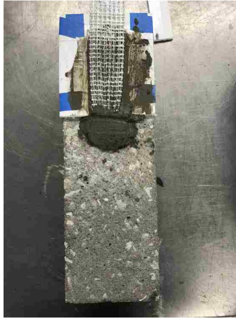
Figure 3.18. Additional anchor-matrix material placement (mortar anchor shown, epoxy anchor similar)
