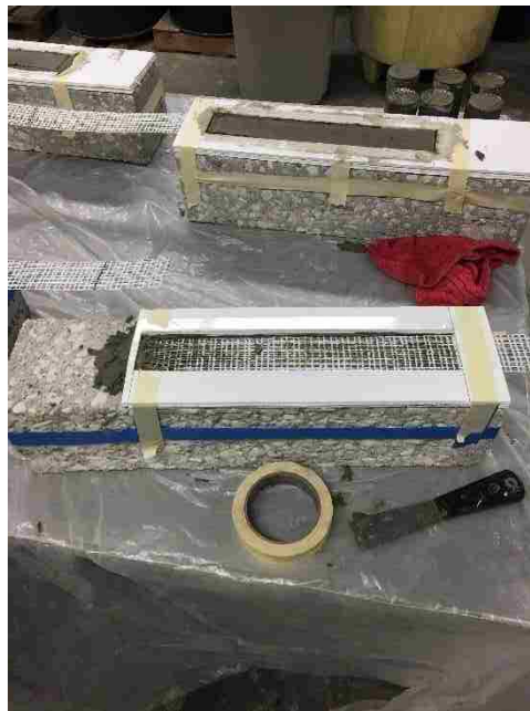
Figure 3.11. Second (external) form secured to concrete prism (anchored specimen shown, control specimen similar)
