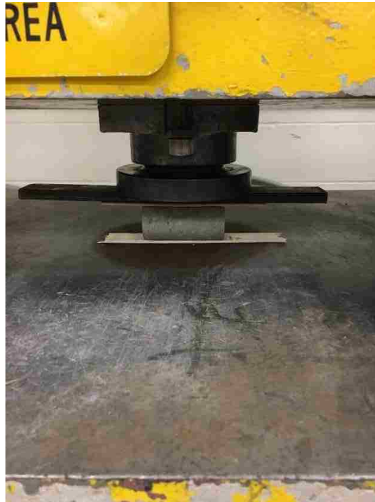
Figure 3.5. Splitting tensile strength test setup
