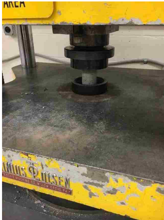
Figure 3.4. Compressive strength test setup
