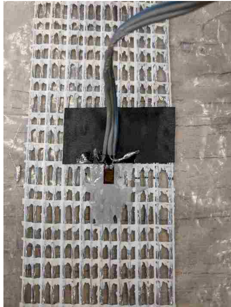
Figure 3.28. Strain gauge with external leads
