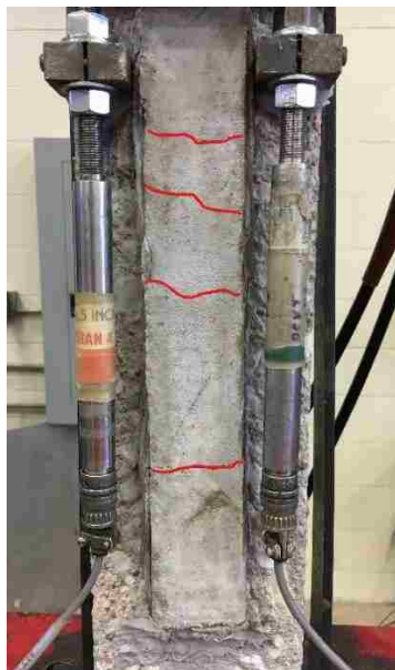
Figure 4.8. Transverse crack pattern for typical anchored specimen (specimen DS_330_50_E_3 shown, transverse cracks shown in red)
