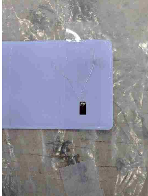
Figure 3.26. Strain gauge prepared for installation
