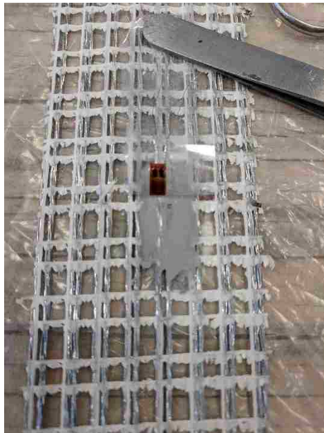
Figure 3.27. Application of accelerant to strain gauge
