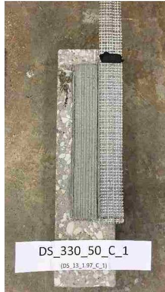
Figure 4.7. Failure of control specimen DS_330_50_C_1
