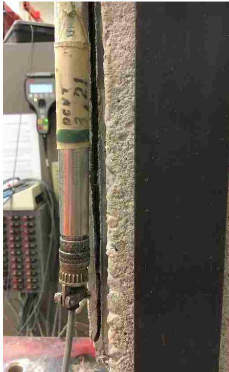
Figure 4.11. Complete debonding of steel fiber at failure (specimen DS_330_50_E_4)
