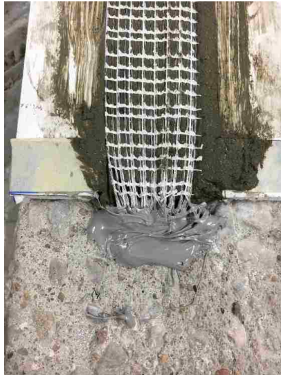
Figure 3.21. Detail of epoxy anchor
