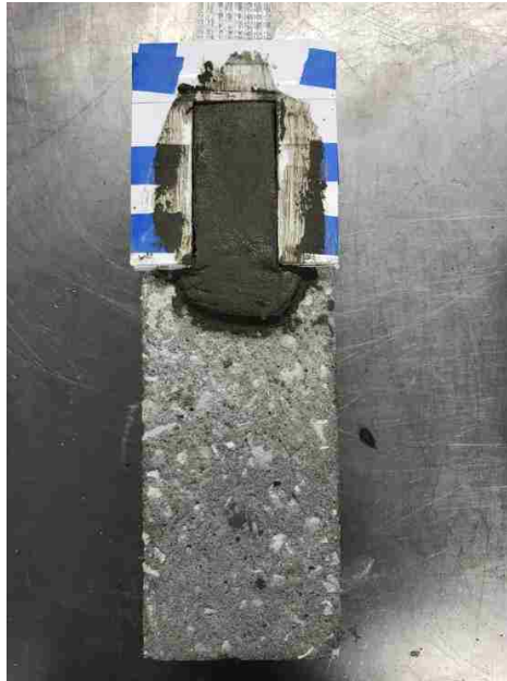
Figure 3.20. External matrix layer application (100 mm bond length shown, 330 mm bond length similar)
