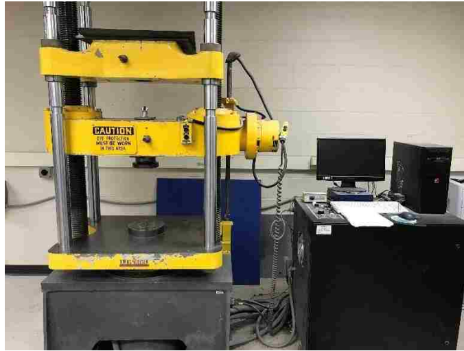
Figure 3.2. Load frame used for concrete and mortar testing
